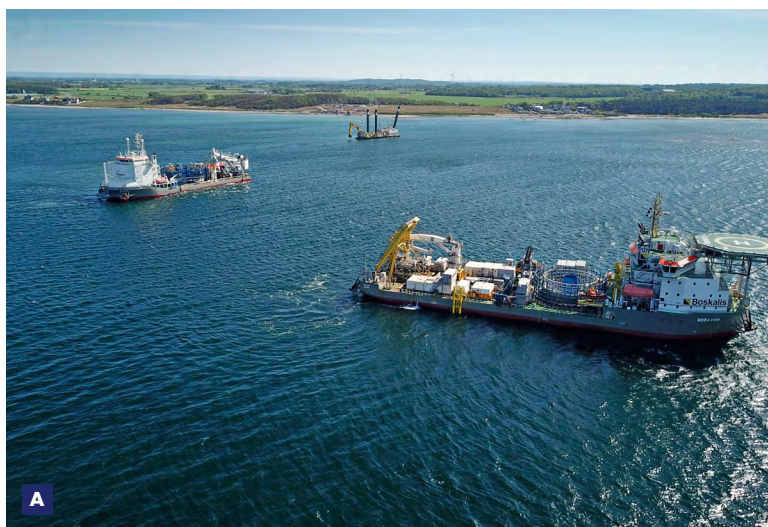
A Boskalis fleet at work: cable burial vessel Ndurance, cable lay vessel Spirit and backhoe dredger Nordic Giant captured in one picture. B Nearshore and Onshore situation
