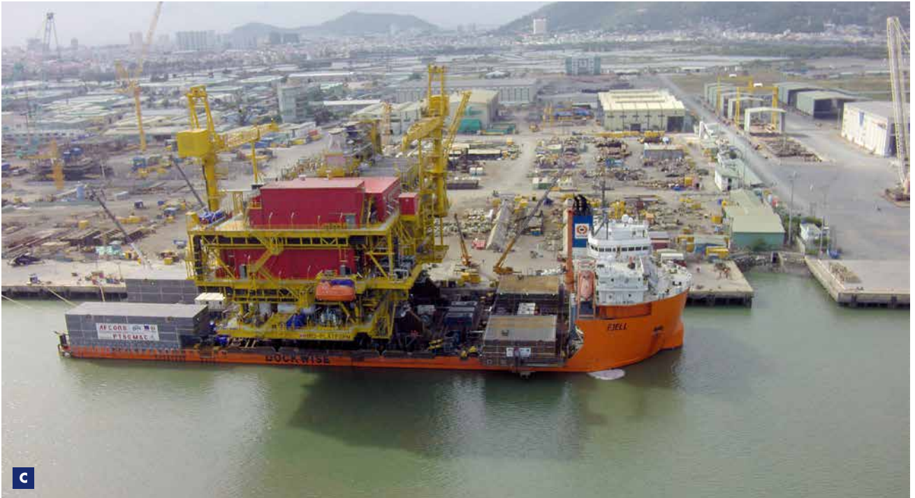
C Loading and transport of the HRD topside onboard the Fjell
