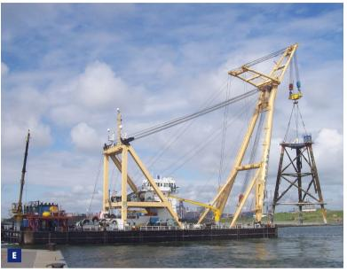
and jacket were transported to the disposal yard in Flushing and offloaded by onshore crawler crane.
