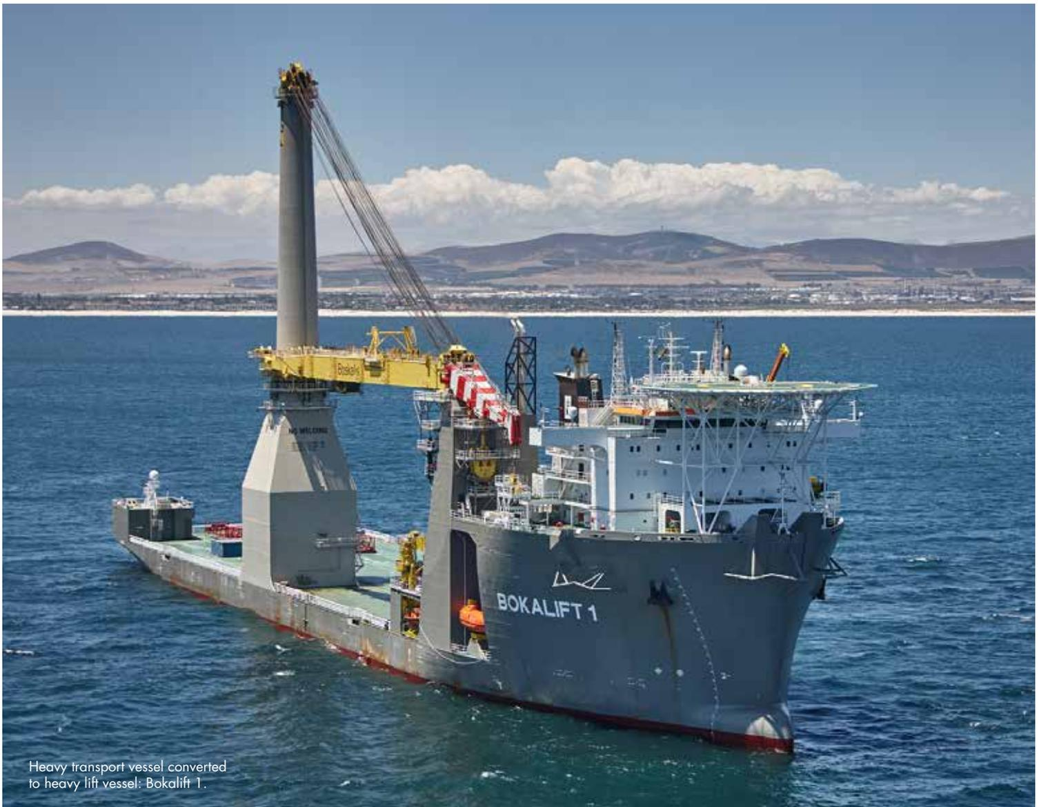
Heavy transport vessel converted to heavy lift vessel: Bokalift 1.
