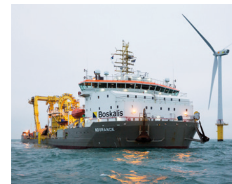
3 MULTI PURPOSE / CABLE-LAYING VESSELS Up to 7,500 DWT 5,000 t turntable capacity
