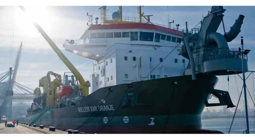
Sustainability was a major feature in designing the trailer hopper suction dredger Willem van Oranje. Ballast water is cleaned before being pumped overboard and space has been reserved for equipment to clean the exhaust fumes even more effectively
