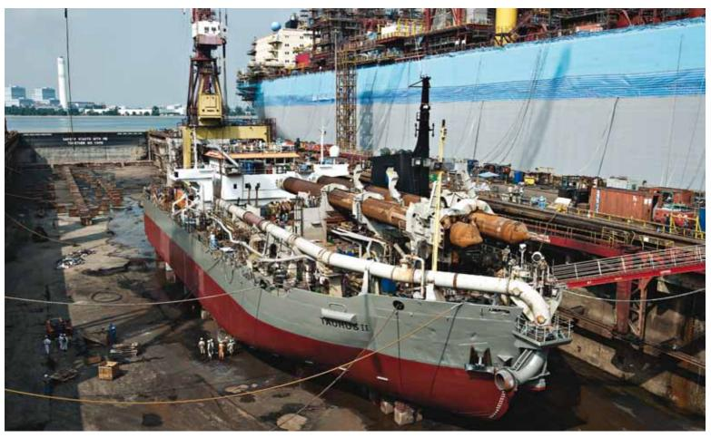
The cutter suction dredger Taurus II at the yard in Singapore where the vessel underwent an overhaul to enable it to sail more efficiently, safely and sustainably
