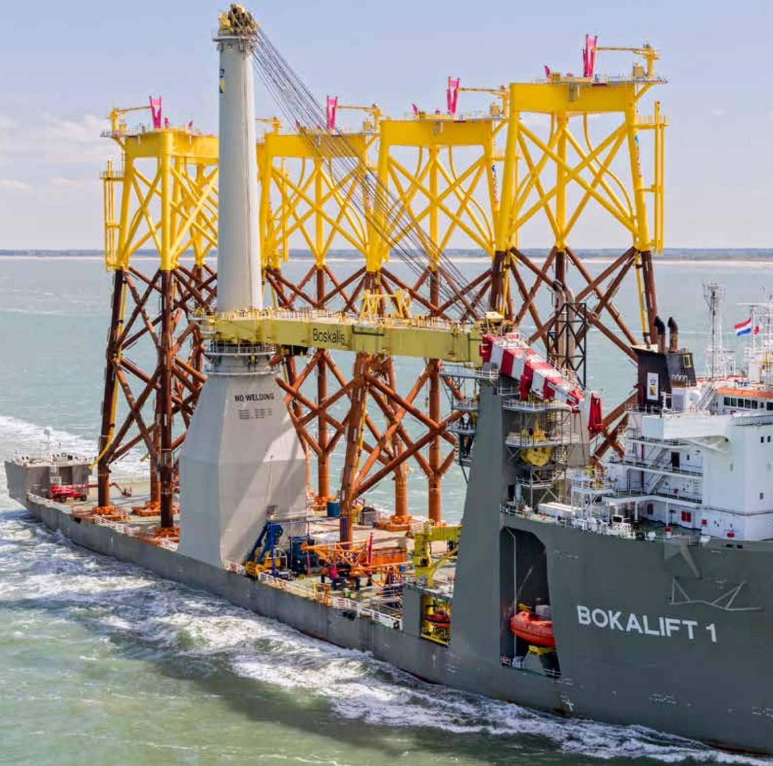
The Bokalift 1 demonstrating its unique capabilities by transporting and installing five giant foundations in one go for the East Anglia wind farm
