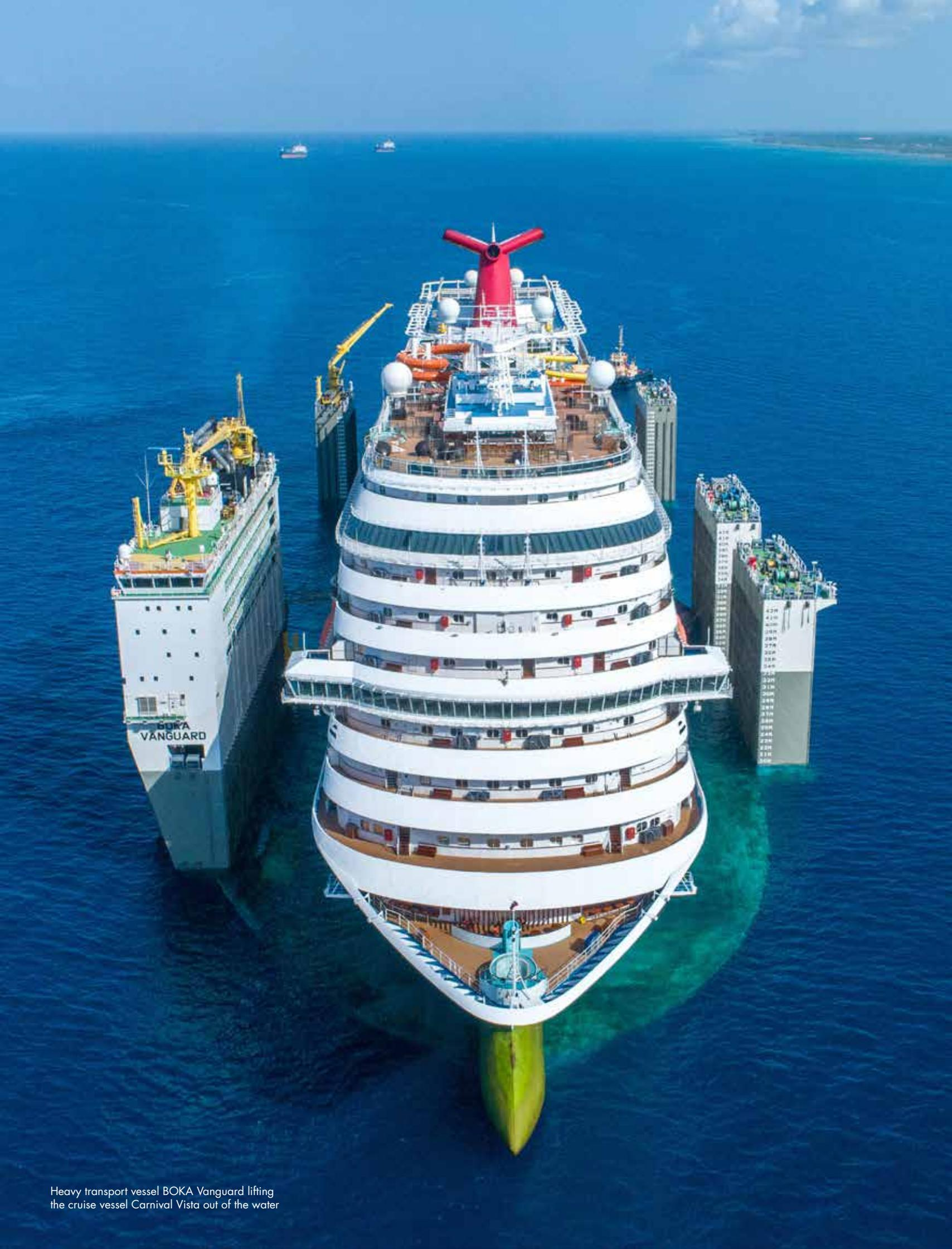
Heavy transport vessel BOKA Vanguard lifting the cruise vessel Carnival Vista out of the water
