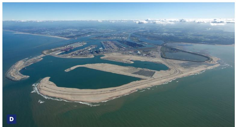
210 million m<sup>3</sup> of sand from the offshore borrow area (located at some 12 km away) to the project site. Four CSDs have been used to dredge the entrance to Maasvlakte 2 from the YangtzeHarbour, to deepen the Yangtze Harbour and to deepen the new port basins to – 20 m and to pump the 30 million m<sup>3</sup> of sand involved to the new harbor areas. The new land is raised to 5 m above NAP.
