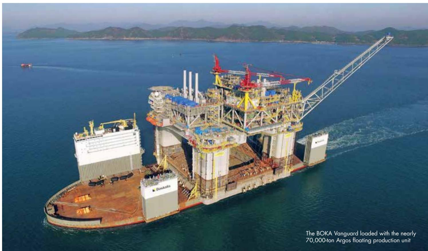
The BOKA Vanguard loaded with the nearly 70,000-ton Argos floating production unit
