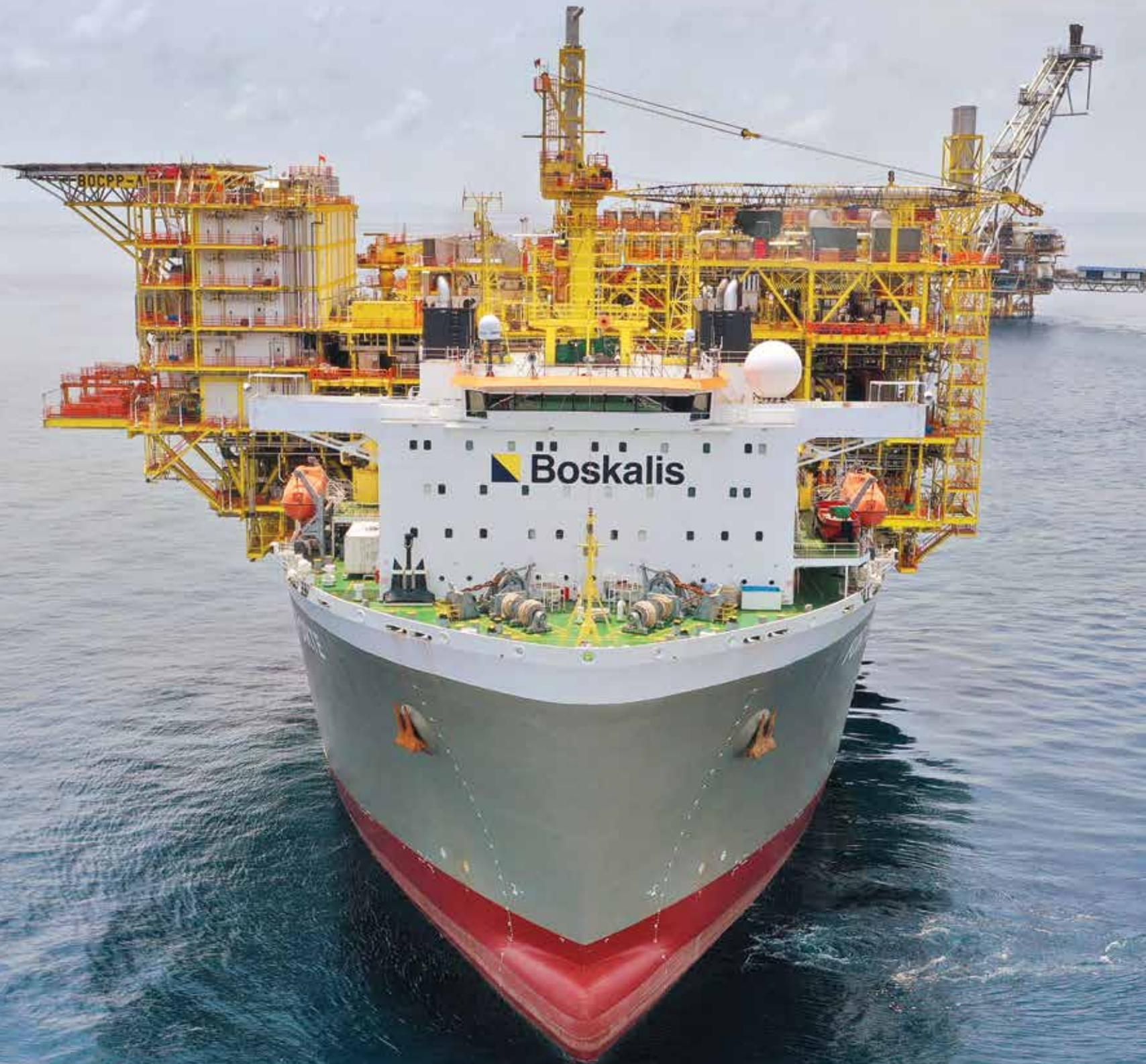
Heavy transport vessel Forte loaded with the 11,500-ton Bokor CPP-A platform topside
