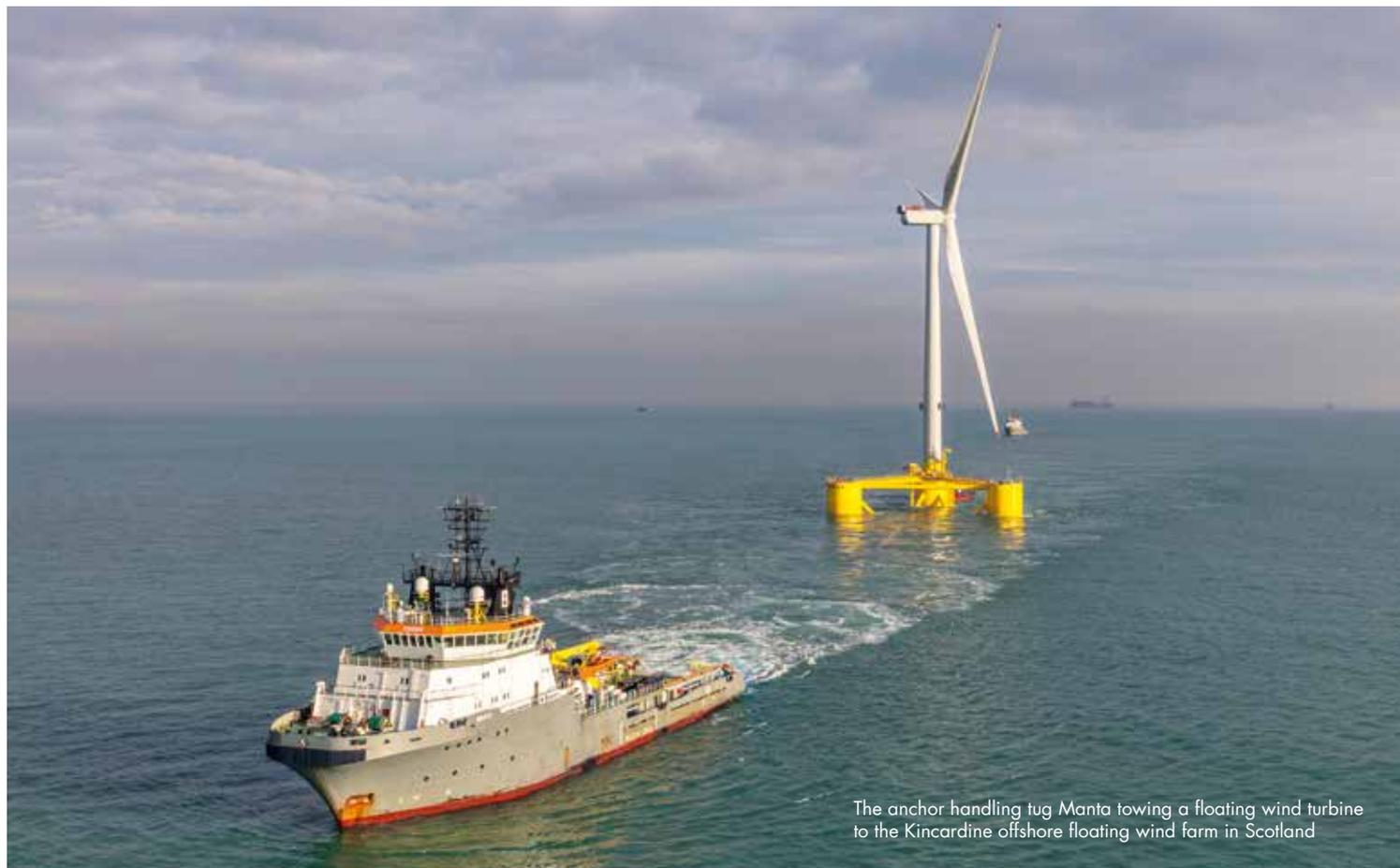
The anchor handling tug Manta towing a floating wind turbine to the Kincardine offshore floating wind farm in Scotland
