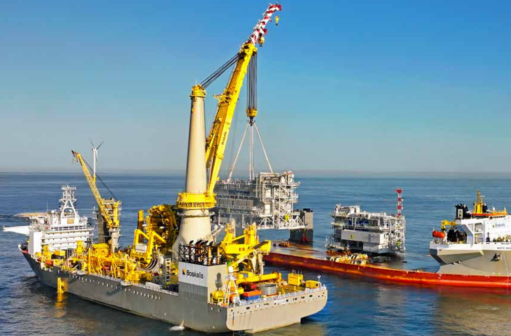
The crane vessel Bokalift 2 lifting a platform topside from the deck of the semi-submersible heavy transport vessel White Marlin
