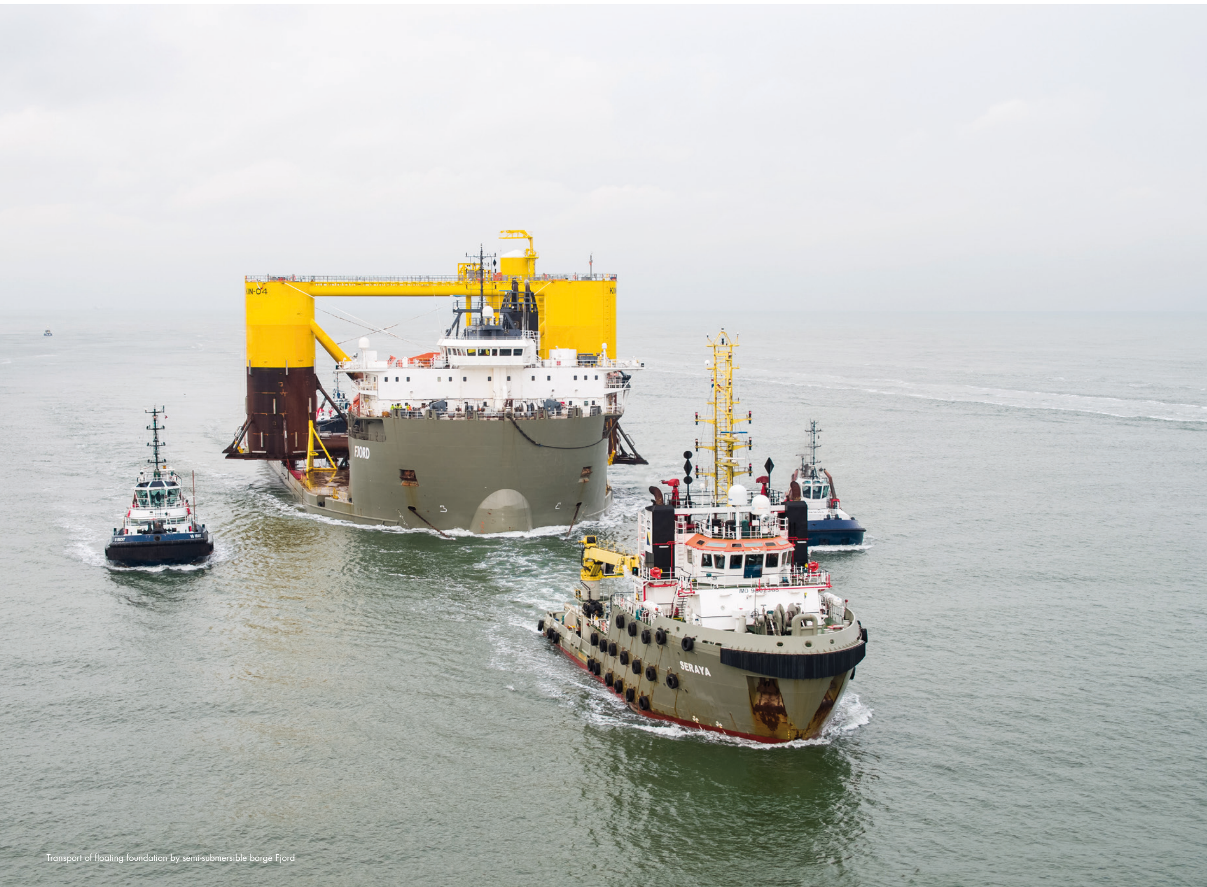
Floating foundation being submerged by semi-submersible barge Fjord
