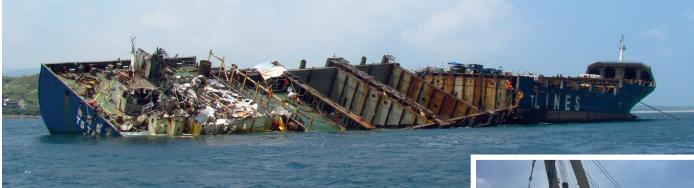
Craig Erasmus (Project Manager) and his team have been working on the wreck removal of the TS Taipei, a container vessel that grounded on a rocky seabed off the north coast of Taiwan, and subsequently broke into two sections. They discharged remaining containers, and cut and lifted the accommodation block and main engine from the wreck. Finally the two sections were refloated and delivered to shore for further scrapping.
