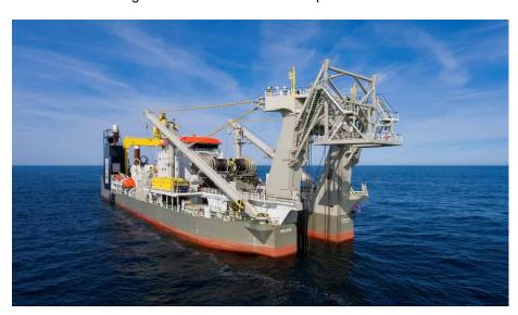
The self-propelled Helios is 152 meters long and has a breadth of 28 meters and is able to dredge at depths of 6 to 35 meters. With a total installed power of almost 24,000 kW, a total pumping capacity of 15,600 kW and a maximum cutter power of 7,000 kW, the Helios is one of the most powerful cutter suction dredgers in the dredging industry. The vessel was developed to dredge in extremely hard ground. The cutter ladder weighs 2,060 tons, making it the heaviest in the world.
