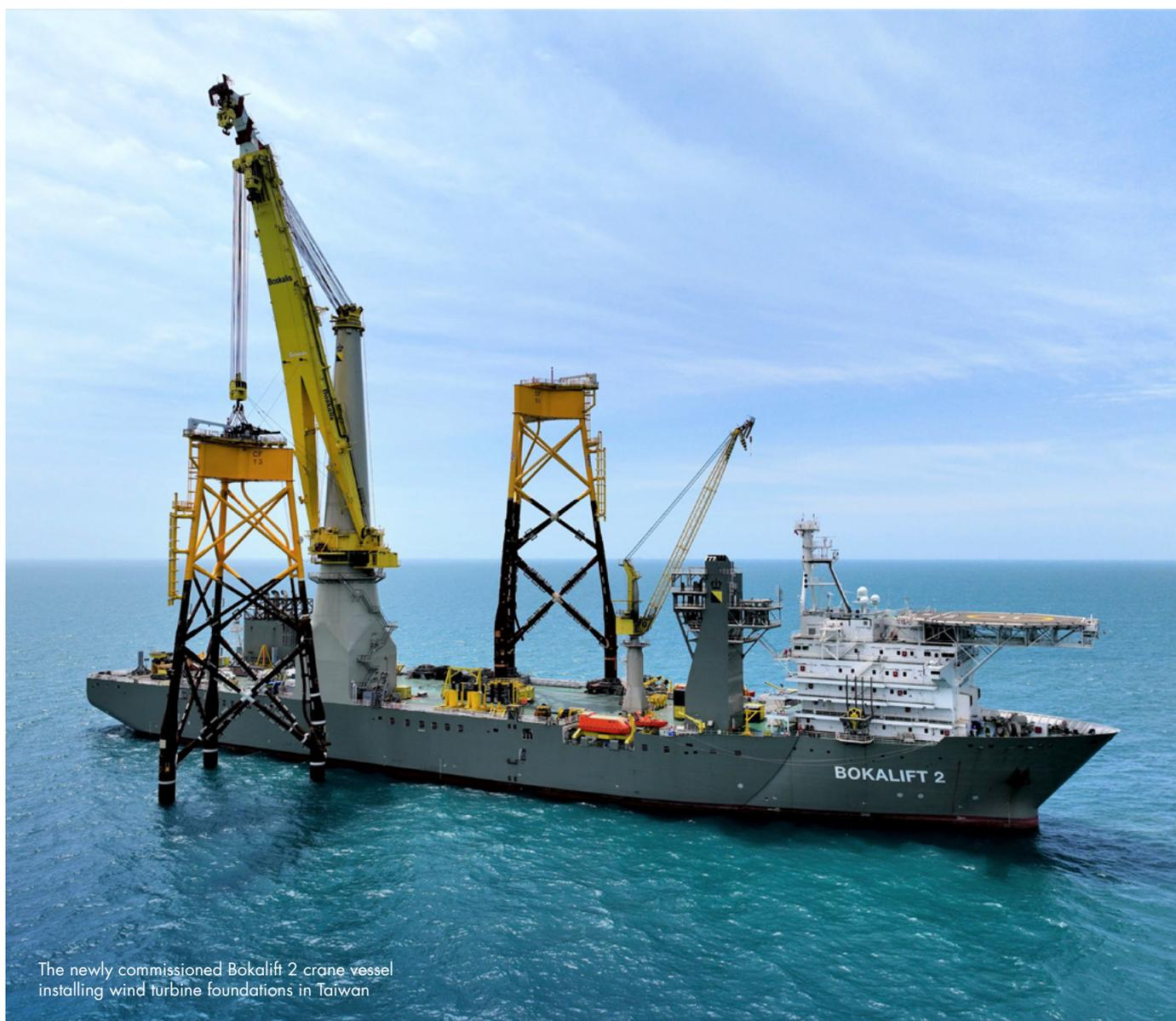
The newly commissioned Bokalift 2 crane vessel installing wind turbine foundations in Taiwan
