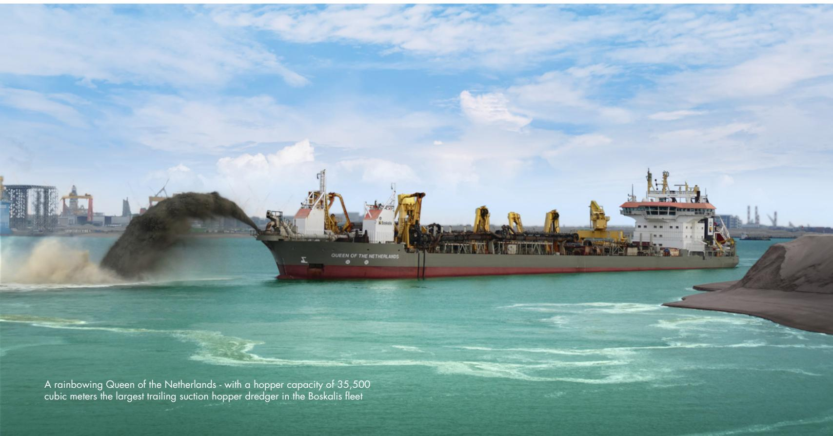
A rainbowing Queen of the Netherlands - with a hopper capacity of 35,500 cubic meters the largest trailing suction hopper dredger in the Boskalis fleet
