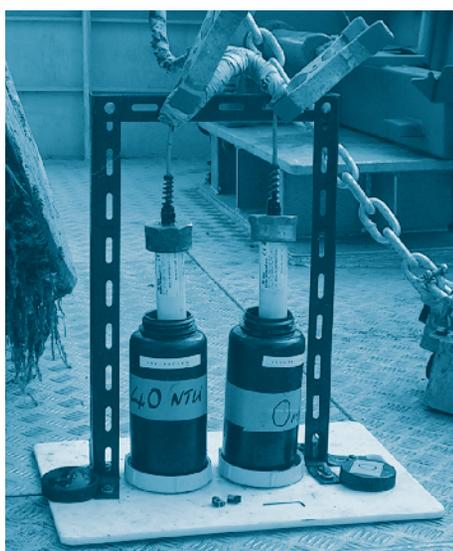
Figure 12. The verification of two turbidity probes.
