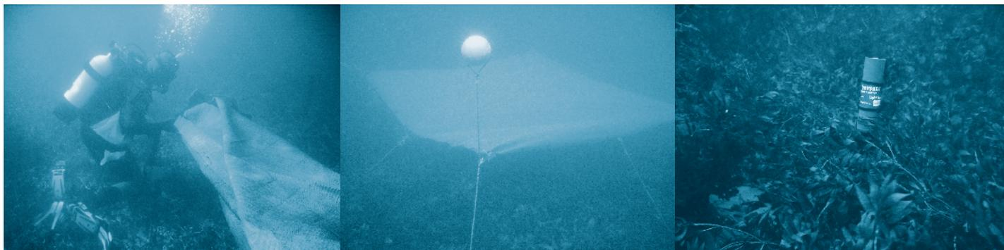
Figure 11. Shading experiments were conducted to determine the impact of biological response to reduced light. From left to right: the installation of a shade, kelp under a shade and a light meter.
