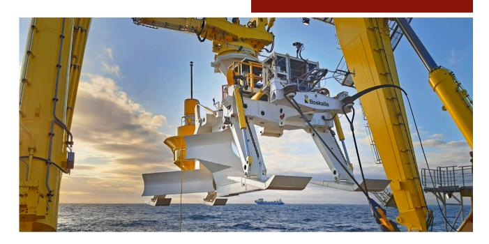
The Megalodon provides our customers with a pre-trench and backfill cable protection solution. The plough can handle up to 150 t continuous pull force and is designed to perform in an extensive range of challenging soil conditions along planned cable routes.
