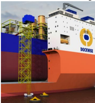
Figure 20: Means of Evacuation
