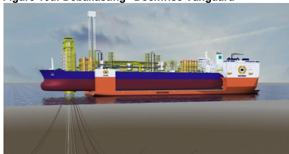
Figure 16e: Dry-docking stage
