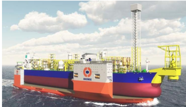
Figure 4: Dry-transport of FPSOs
