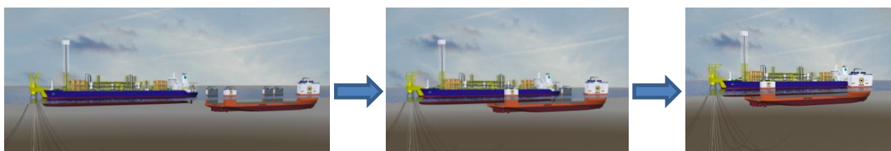
Figure 14: Loading Operation External Turret Moored FPSO
