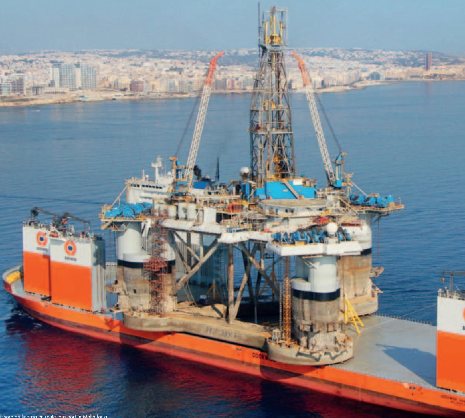
Offshore drilling rig en route to a port in Malta for a dry-docking operation on board of the Dockwise Vanguard
