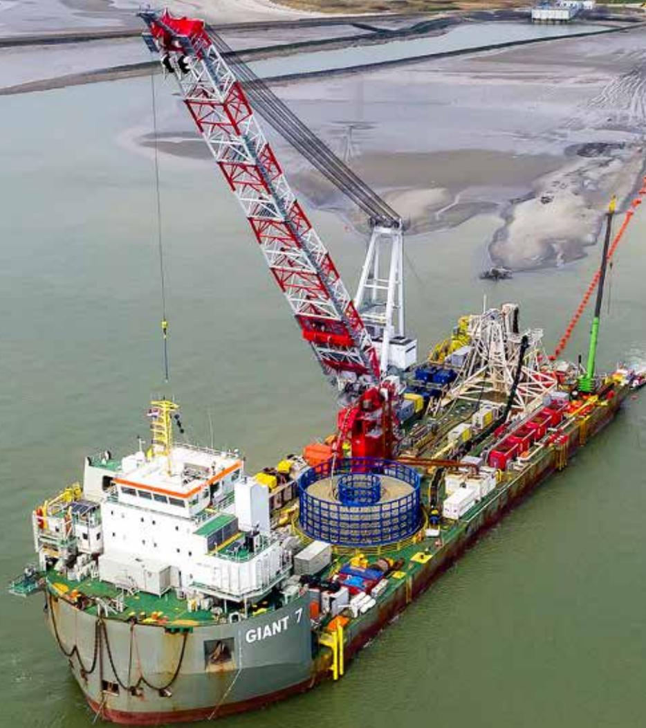
Boskalis is currently completing the installation of the last of the four 220 kV export cables that connect the Borssele offshore wind farms in the North Sea to the high-voltage grid in the Netherlands. "The project is a showcase of versatility and teamwork between various disciplines of our company," project director Hans Veth said.
