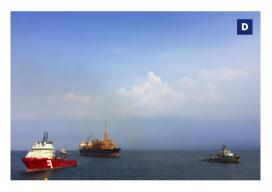
After completion of the mooring installation in Phase 1, the FPSO was towed from Singapore to Madura field for hook-up operations.
