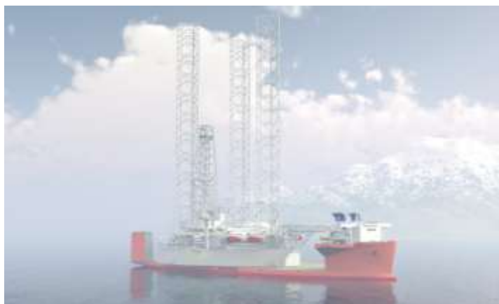
Artist impression of M/V White Marlin carrying a Cat-J size jack-up rig Click here to download a high resolution artist's impression
