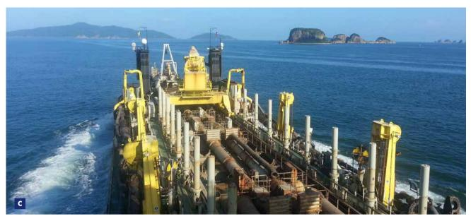
discharged into pusher tug barges for transport to the designated disposal area. The TSHD Cornelis Zanen was deployed in the areas of sufficient depth to deepen the channel and port basin to the required depths and slopes.
