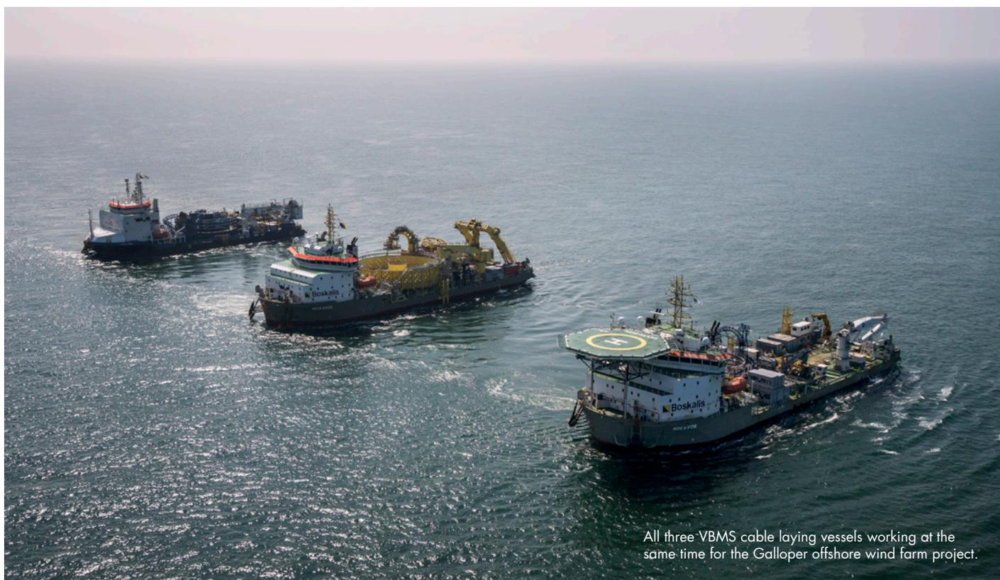
All three VBMS cable laying vessels working at the same time for the Galloper offshore wind farm project.
