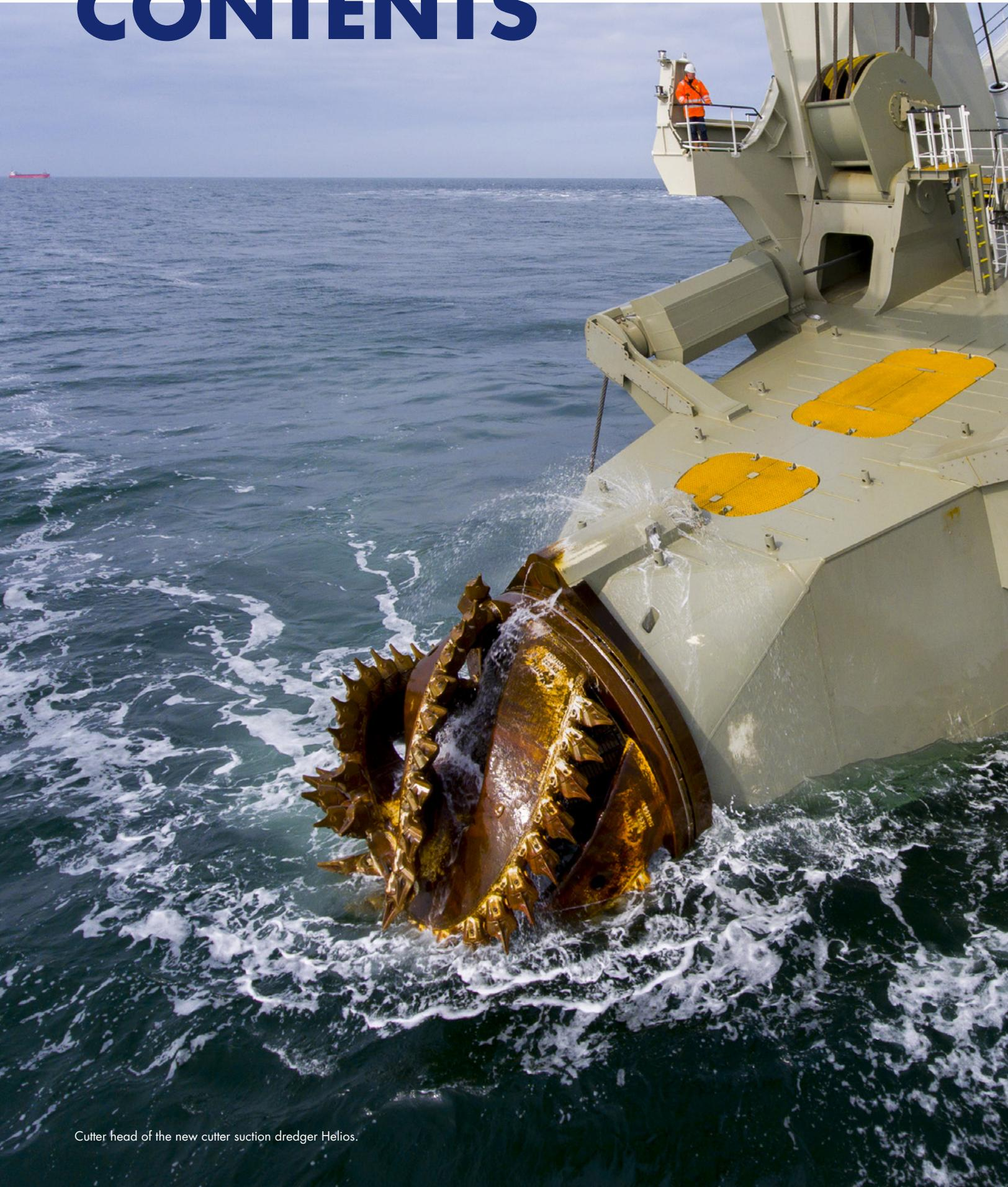
Cutter head of the new cutter suction dredger Helios.
