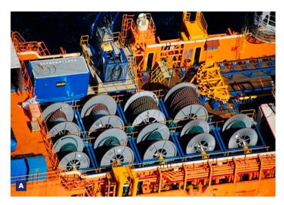
The second installation spread consisted of a purpose-built reel drive cable installation spread that was installed on the rear deck of the DP2 offshore construction vessel, Toisa Wave. This vessel ran into port to load 9 cable drums at a time. This set-up proved to be extremely efficient, resulting in the timely completion of the cable installation scope, ahead of schedule.
