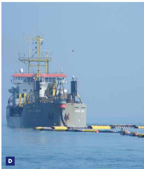
D TSHD Barent Zanen backfilling at Denia E Pipe pull at Mallorca
