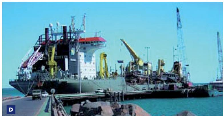
900,000 cubic metres of material in water depths up to 55 metres. Within three weeks, the works were executed by the Trailing Suction Hopper Dredger "Queen of the Netherlands" in challenging conditions of offshore working environment, seabed soils, strict technical specifications and the sensitive underwater environment. This demanded thorough preparation of vessel, crew and clear working procedures to guarantee safe, sound and efficient completion of this part of the job.
