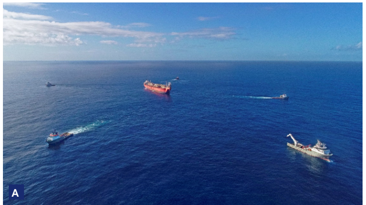
A The Station keeping of FPSO Fluminense with 4 tugs and Boka Falcon ready to cut a mooring line
