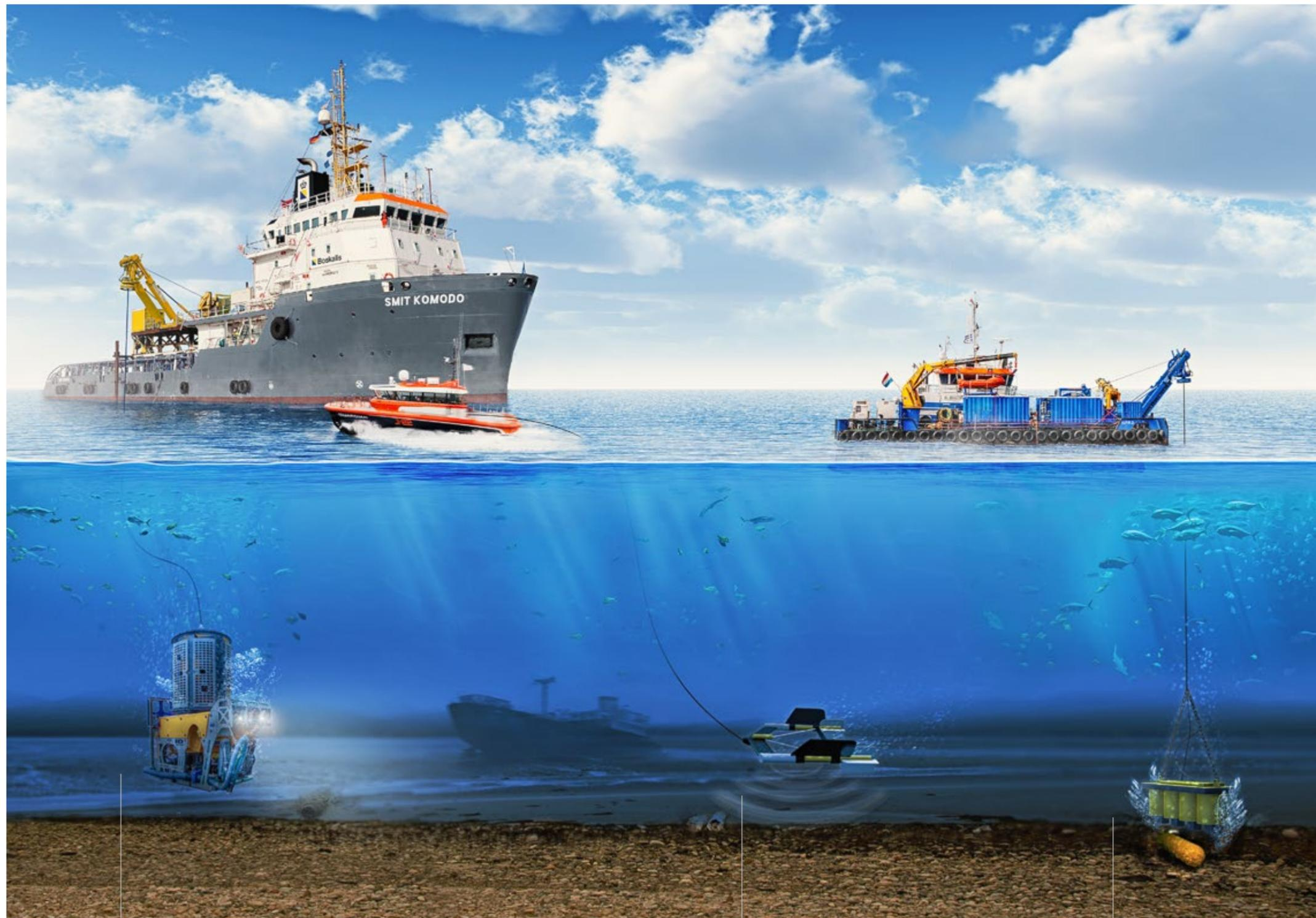
Heavy-Duty Work Class Remotely Operated Vehicle (HD-WROV) for locating and salvaging ammunition
