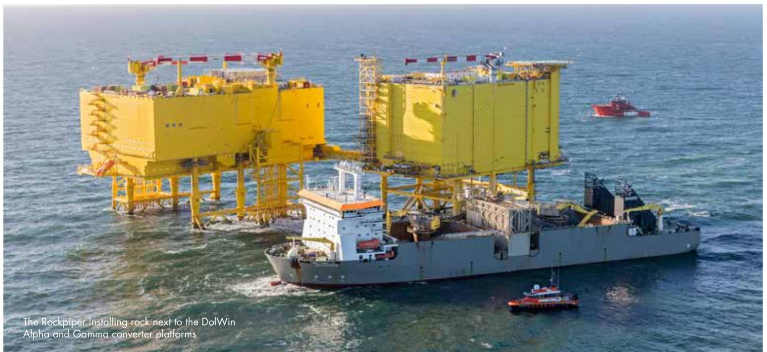
The Rockpiper installing rock next to the DolWin Alpha and Gamma converter platforms
