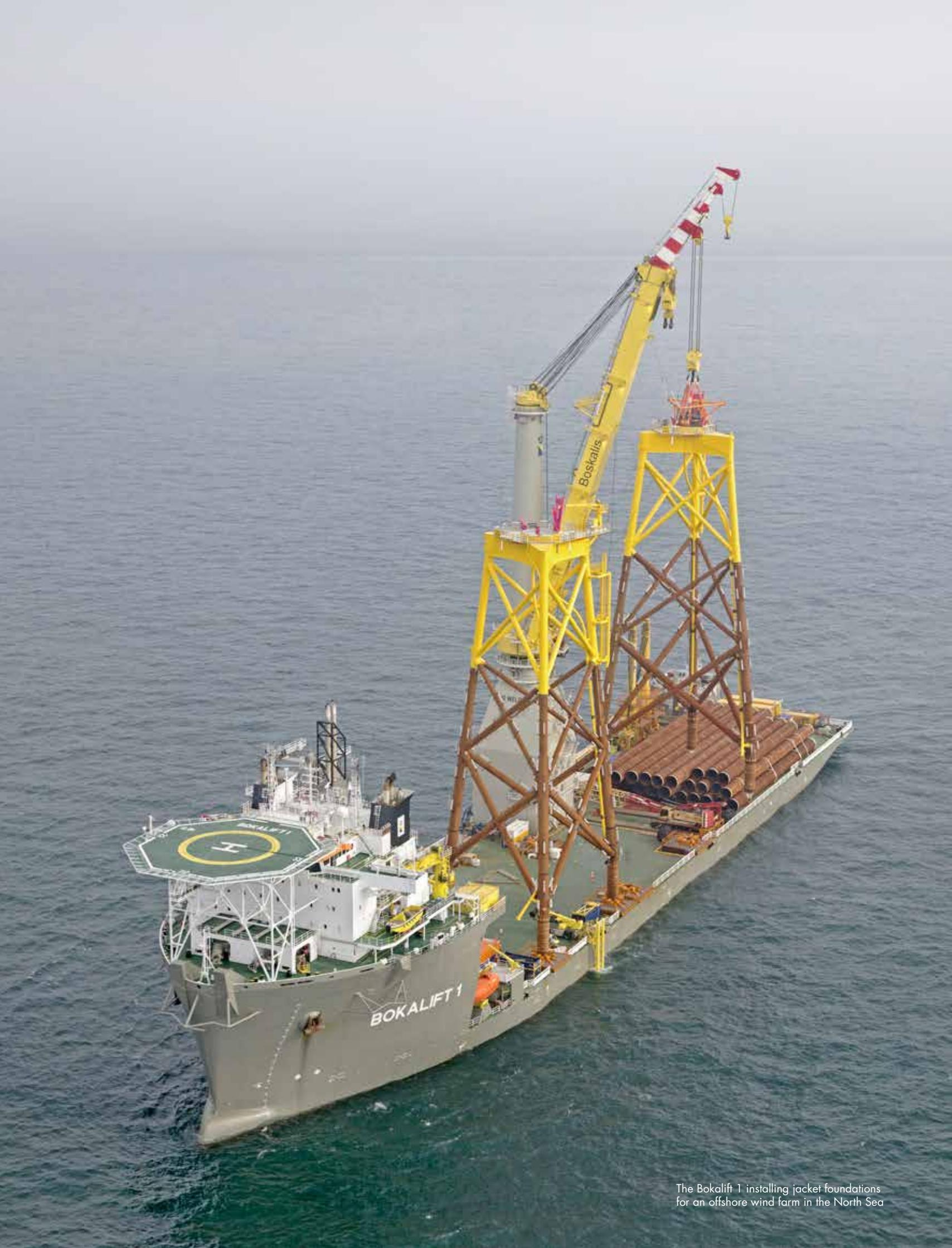
The Bokalift 1 installing jacket foundations for an offshore wind farm in the North Sea
