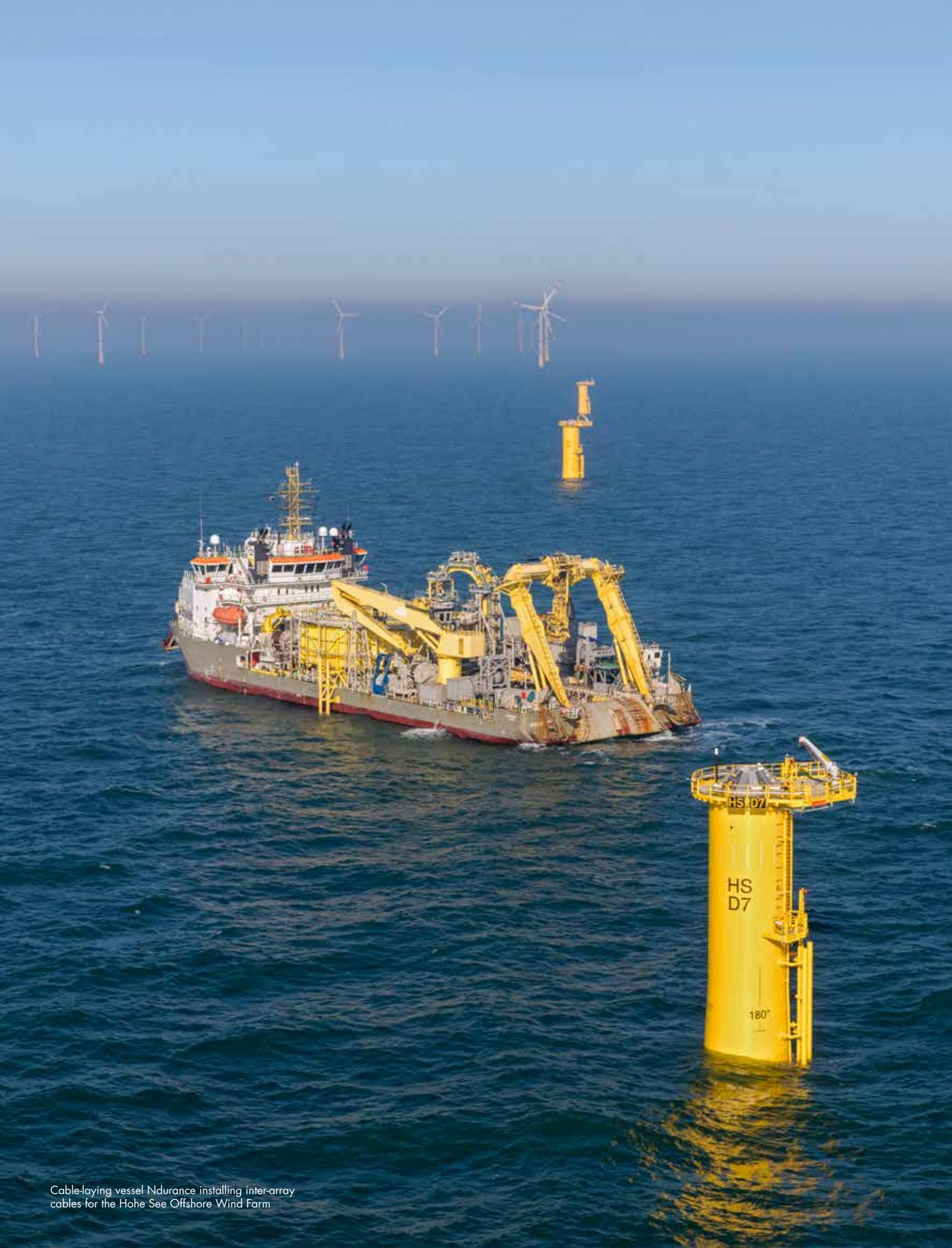
Cable-laying vessel Ndurance installing inter-array cables for the Hohe See Offshore Wind Farm
