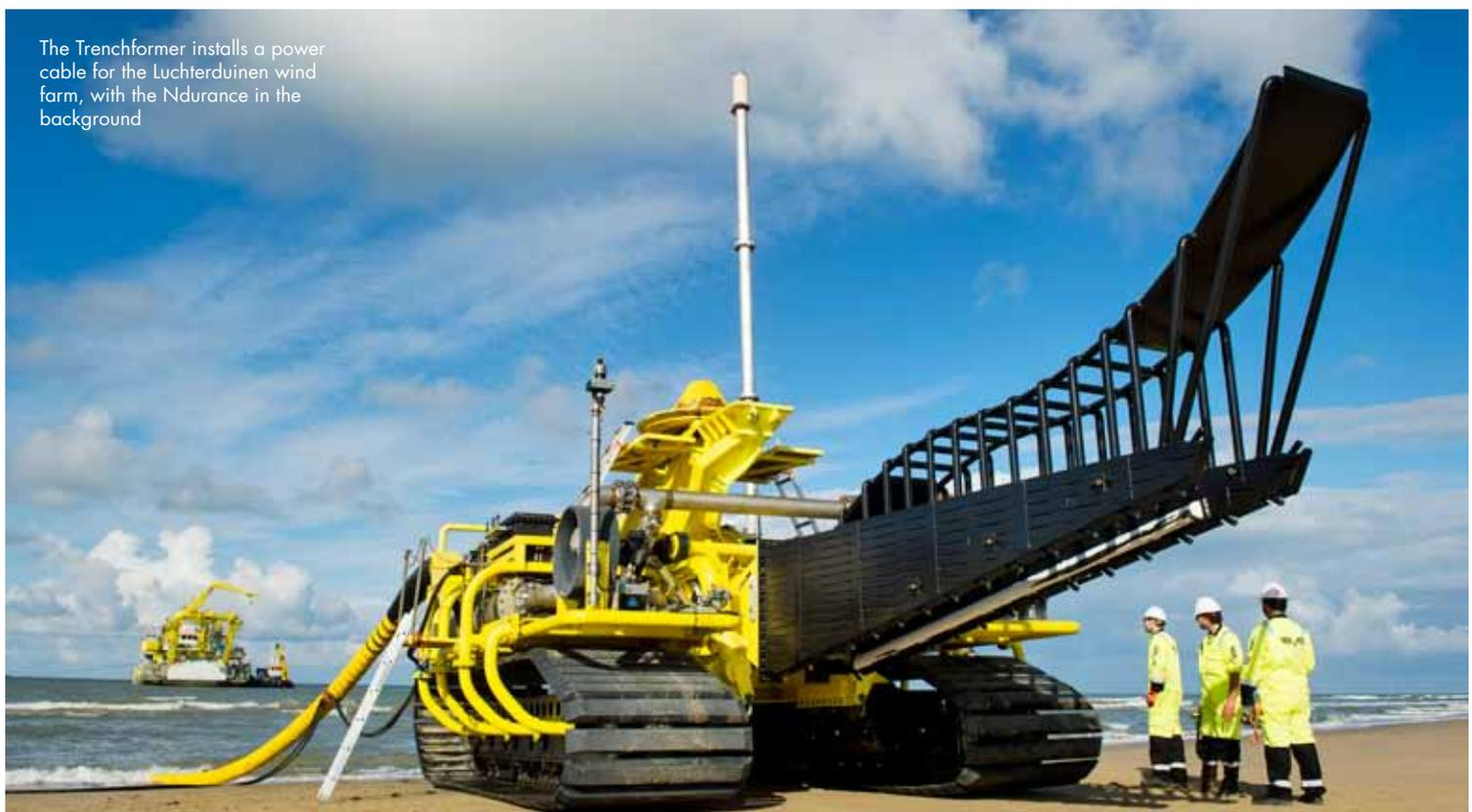
The Trenchformer installs a power cable for the Luchterduinen wind farm, with the Ndurance in the background
