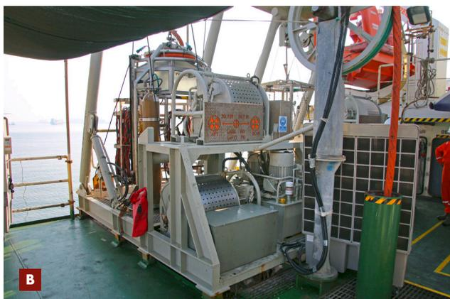
Air dive spread 38 is a modular, containerized Mixed Gas/Air Diving spread which has been designed for swift mobilization and demobilization onto/ from Boskalis or client- supplied vessels, platforms or Rigs.
