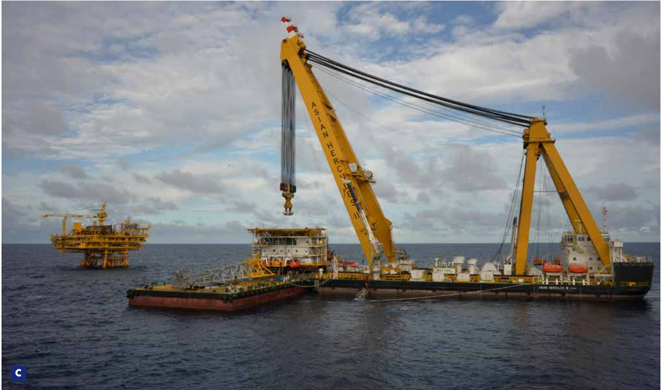
C Asian Hercules III preparing to lift Living Quarters of cargo barge
