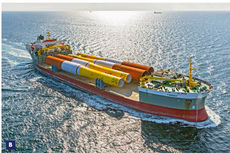
A MP installation on SFW B Transportation of MP's
