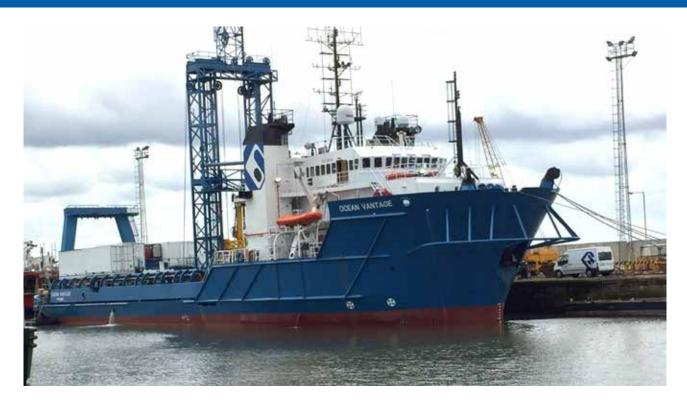
MV Ocean Vantage is a DP2 geotechnical vessel offering a range of drilling, in situ testing, laboratory testing and sampling services through a central moonpool or via the vessel's 15-tonne stern A-frame.
