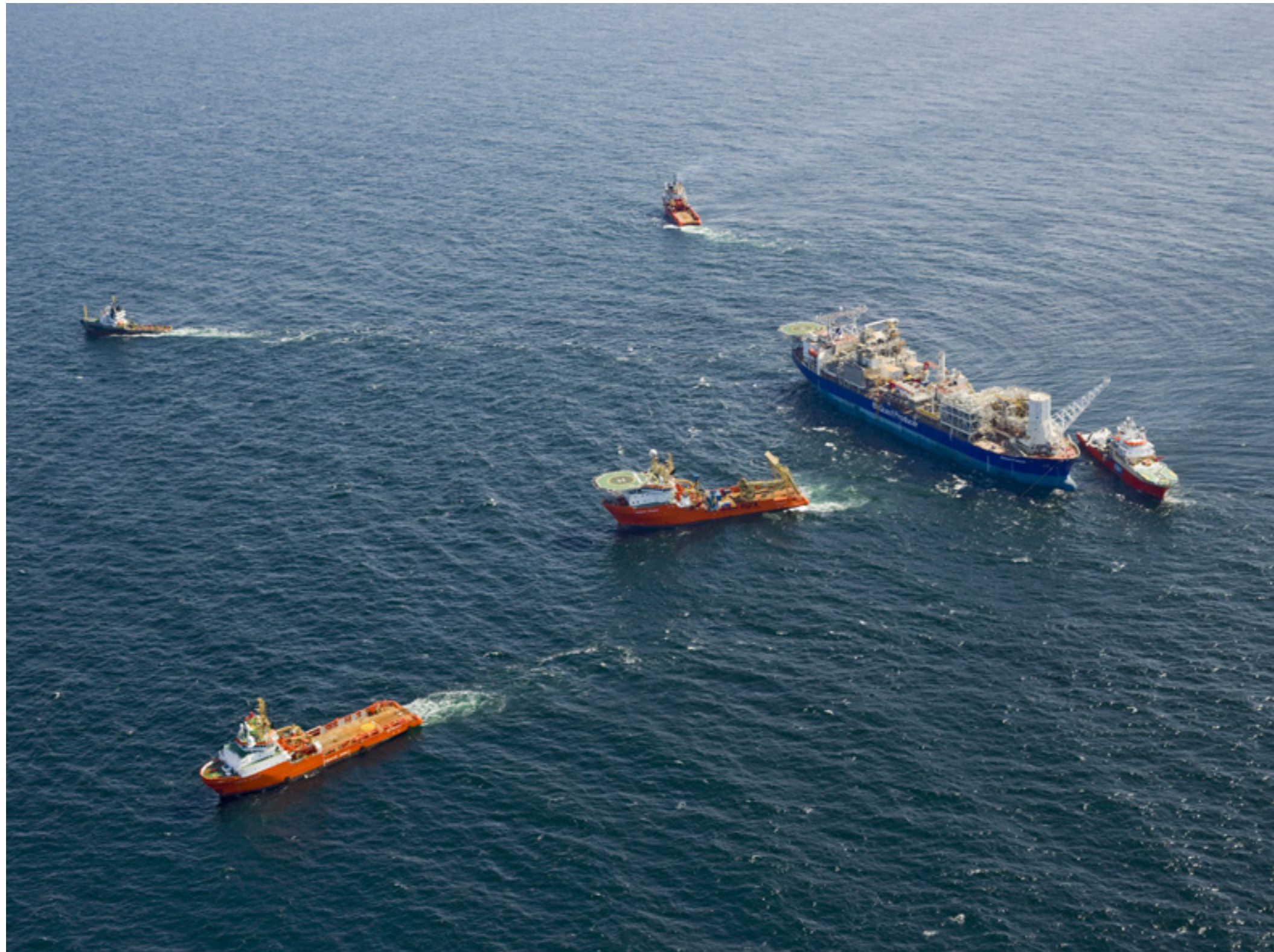
UNITED KINGDOM Enquest Producer Mooring System & Riser Hook-up with DSV EDT Protea and various assisting AHTs.
