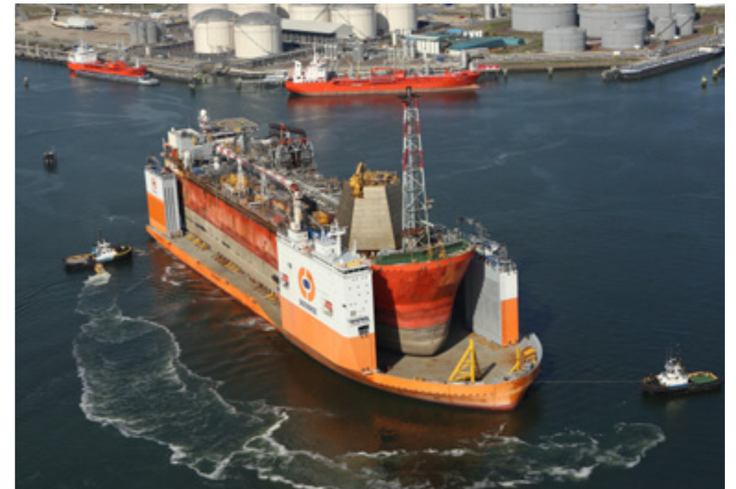
THE NETHERLANDS - INDONESIA Dry-transport of the FPSO Armada Intrepid onboard the Dockwise Vanguard.
