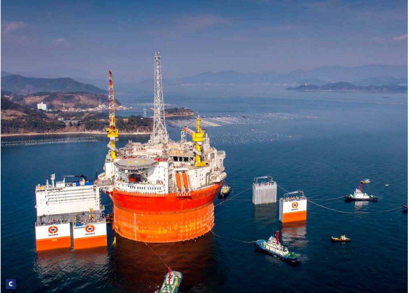
C The Dockwise Vanguard submerged loading the Goliat FPSO.
